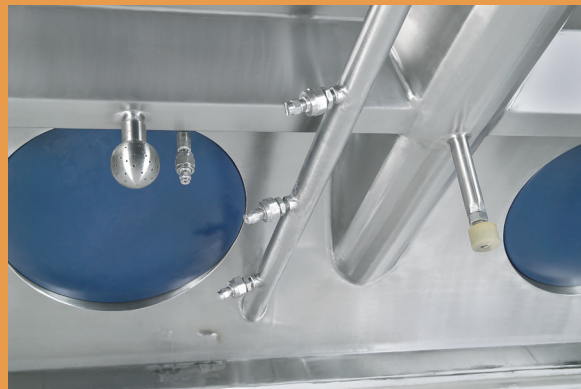
Clean-in-place system contained in cover
